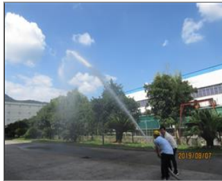
External photo(s) of the production unit(s) Fire hydrant testing.JPG
