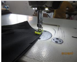
External photo(s) of the production unit(s) 7.17 No needle guard was installed.JPG
