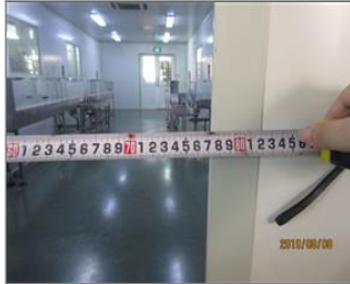
External photo(s) of the production unit(s) 7.15 The width of exit was less than the national standard.JPG
