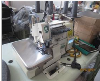
External photo(s) of the production unit(s) 7.17 No eye shield was installed.JPG
